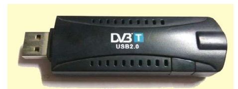
Figure 2 - A DVB-T dongle with RTL2832U, RTL820T or RTL820T2 chipset for reception.
