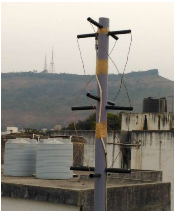
Figure 3 – VU2MIB homebrew QFH antenna for NOAA reception
