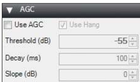
Figure 12 - The Automatic Gain Control Panel
