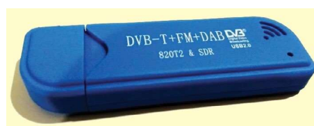
Figure 2 - A DVB-T dongle with RTL2832U, RTL820T or RTL820T2 chipset for reception.
